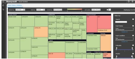
Fault Tree and Asset Status Heat Maps aid in quick identification of priority issues and aid prompt identification of root cause.
