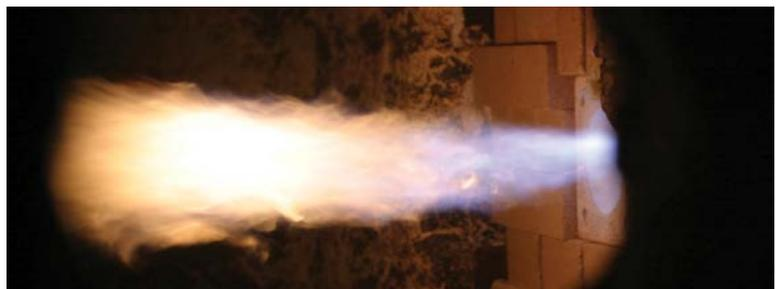
Figure 2: Oxy-Therm LE staged oxygen, conical flame burner.
