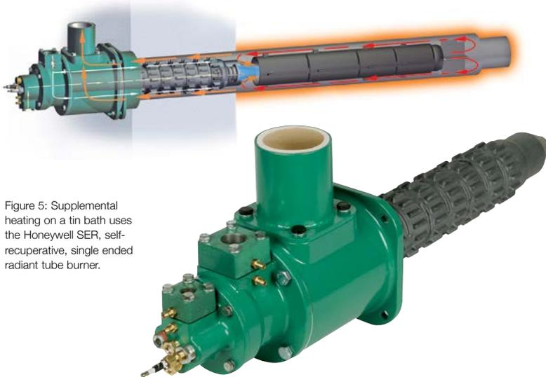
Figure 5: Supplemental heating on a tin bath uses the Honeywell SER, self-recuperative, single ended radiant tube burner.
