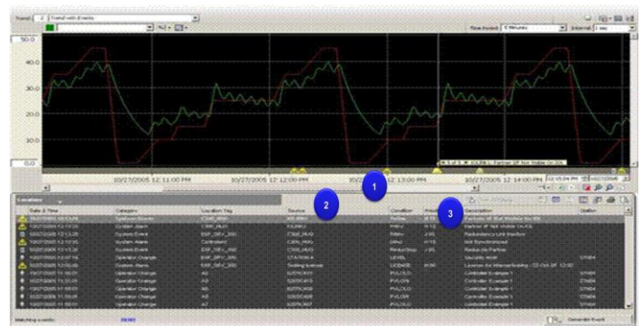
Figure 2. Trend with events is a new trend view that allows operators to correlate and understand the relationship of process events with the process trend/history and to perform extensive analysis of process upsets and disturbances, increasing operator effectiveness. In this sample: ❶ Icons representing each event are shown in a bar below the trend at the point in time the event occurred; ❷ Use the splitter bar to show as much or as little of the event data as necessary; ❸ Clicking on an event puts a hairline on the trend. If more than one event occurred at that point in time, a scrollable tool tip indicates the events. As the operator scrolls through the events, they are highlighted in the event summary as well.
