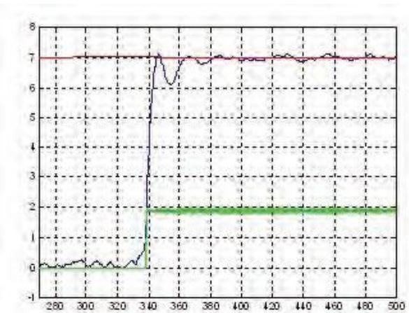
Figure 2 - Start-up mold level control after soft-sensor implementation
