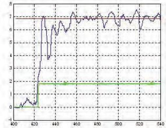
Figure 1 - Start-up mold level control before soft-sensor implementation
