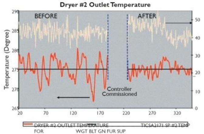
Figure 1 - Comparison of the temperature deviation before and after controller implementation.
