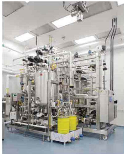
One-Wireless Operator Stations provide remote access to process equipment and reduce the number of user interfaces in sterile process areas.
