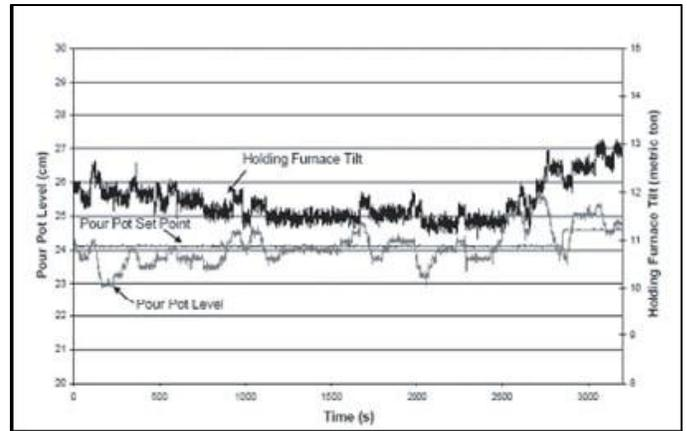
Figure 2- Level deviation after controller implementation
