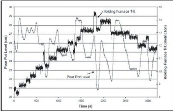
Figure 1- Level deviation before controller implementation
