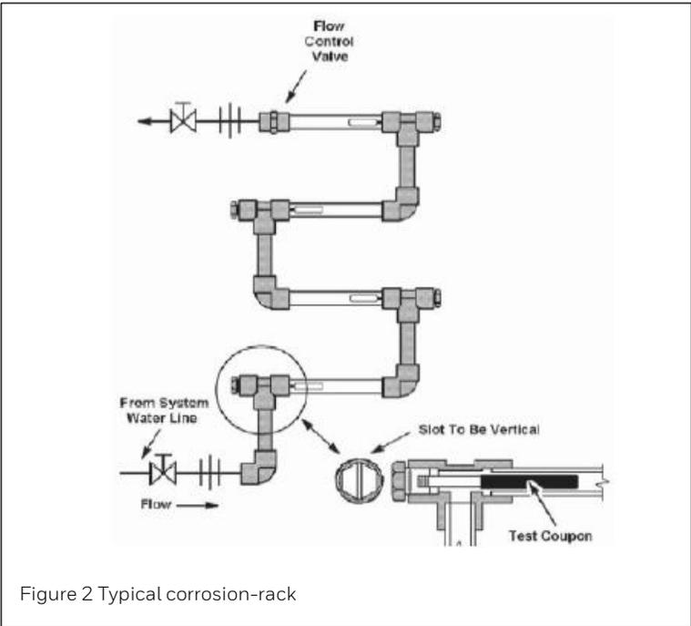
Figure 2 Typical corrosion-rack
