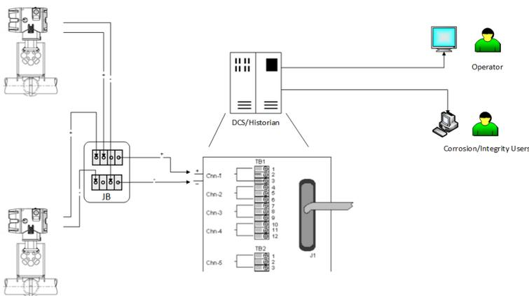
Figure 3 Schematic connection of SmartCET with DCS-HART enabled system
