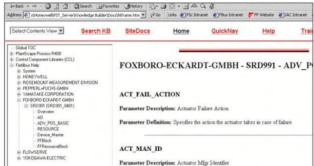
Help information from Device Description files is automatically added to Knowledge Builder and indexed to Control Builder
