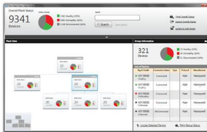
Figure 4. Field Device Manager Plant Area View
