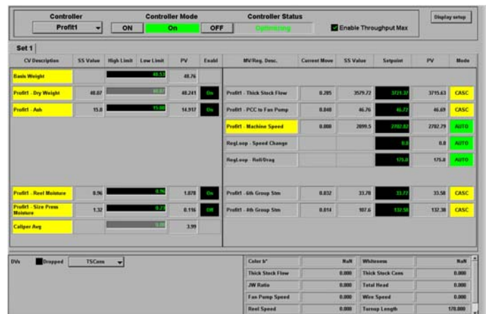
MD Control Summary display with production optimization running
