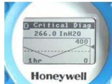
For critical diagnostics, however, the LCD also displays a "Critical Diagnostic" banner, and a message indicating the fault category is included in the screen rotation (above).
