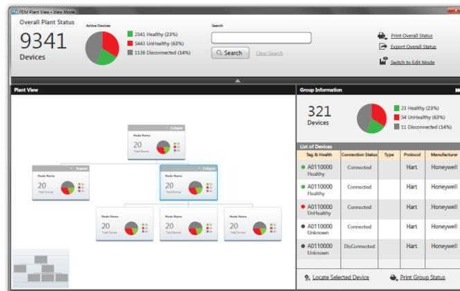
Figure 1: FDM Plant Area View Screen
