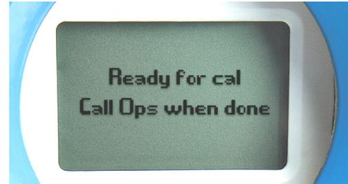
temperature transmitters, even the temperature sensors, have to be maintained efficiently in order to achieve desired results. Temperature sensors in tough applications are maintenance intensive and involve frequent intervention to fix issues relating to open sensor, sensor degradation, etc. Therefore, transmitter messaging is essential in communicating to field operators and enhancing maintenance and safety.
