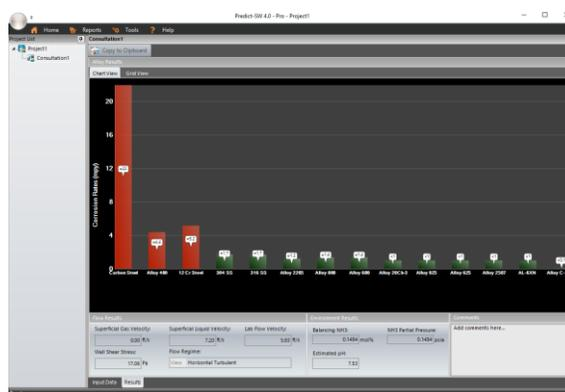
Figure 3: Predict-SW 4.0 program output interface, showing corrosion predictions
