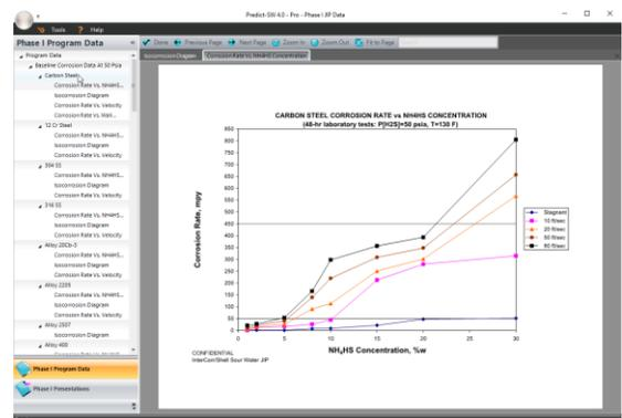
Figure 4: Predict-SW 4.0 JIP data for carbon steel
