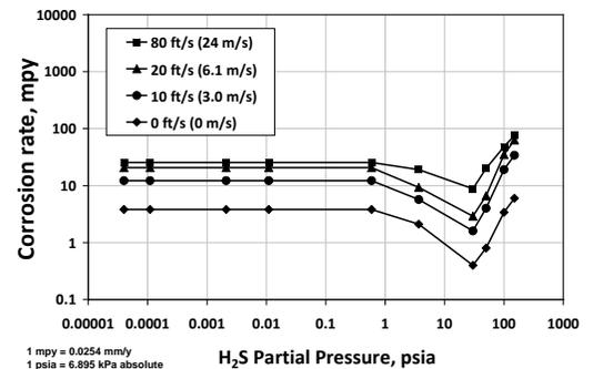
Figure 2: Extensive experimental data correlating corrosion rate to process parameters (Carbon Steel, 1% NH<sub>4</sub>HS, 130 F (55 C))
