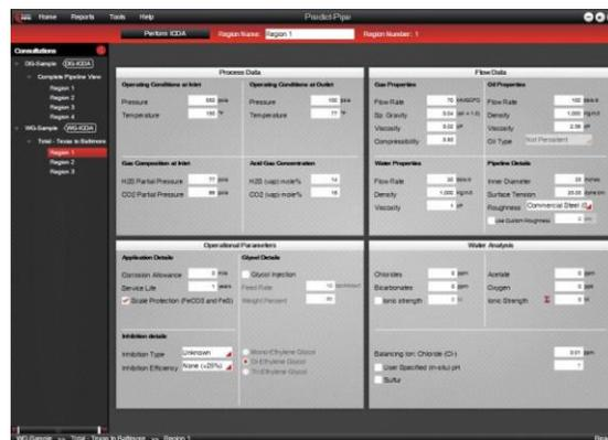
A typical WG-ICDA region input screen in Predict-Pipe
