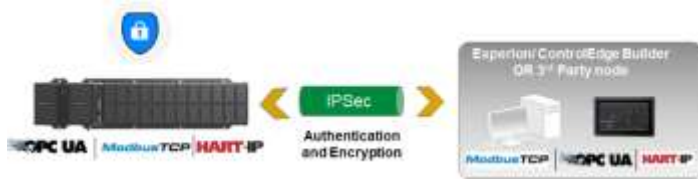
Figure 6. PLC Communication Secured with IPSec
