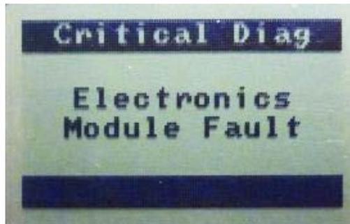
SmartLine STT850 Temperature Transmitter with Advanced Display showing Critical Diagnostic failure (Electronic Module Fault).
