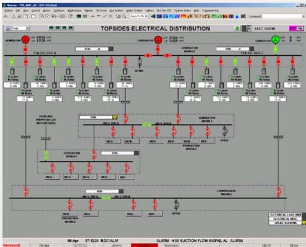
Figure 2, Single-Line Diagram in Experion Station
