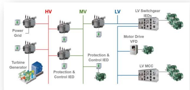
Figure 1, Powering the Process
