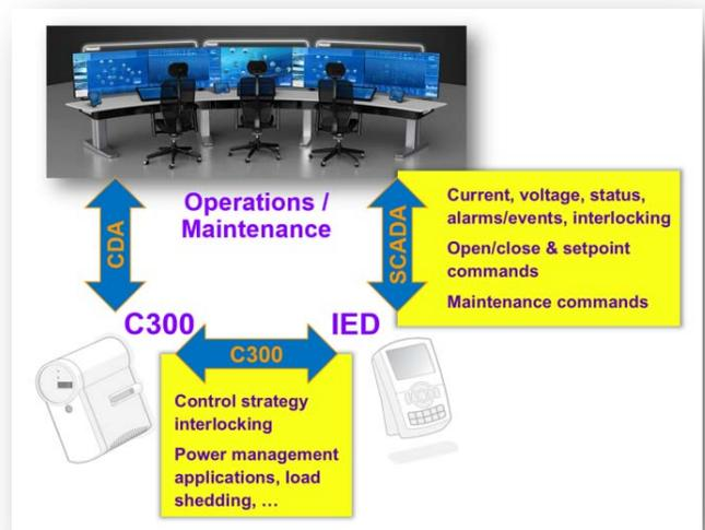
Figure 4, Experion's Flexible Architecture
