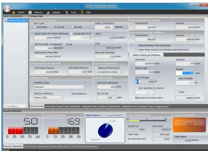
Predict program interface, showing predicted pitting corrosion potential and general corrosion rate for carbon steel
