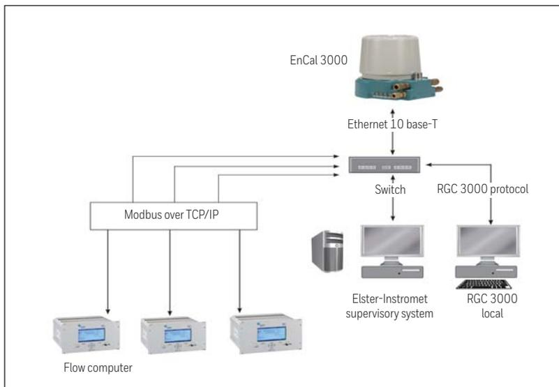
analysis. The EnCal 3000 simply recalculates the analysis results based on the raw data of a previously performed analysis. This is a time-saving option, whenever the operator needs to optimize the analysis. The RGC 3000 software can also be used to update the embedded software of the gas chromatograph, should any new software releases become available. This can be done locally or remotely, provided the EnCal 3000 is connected
