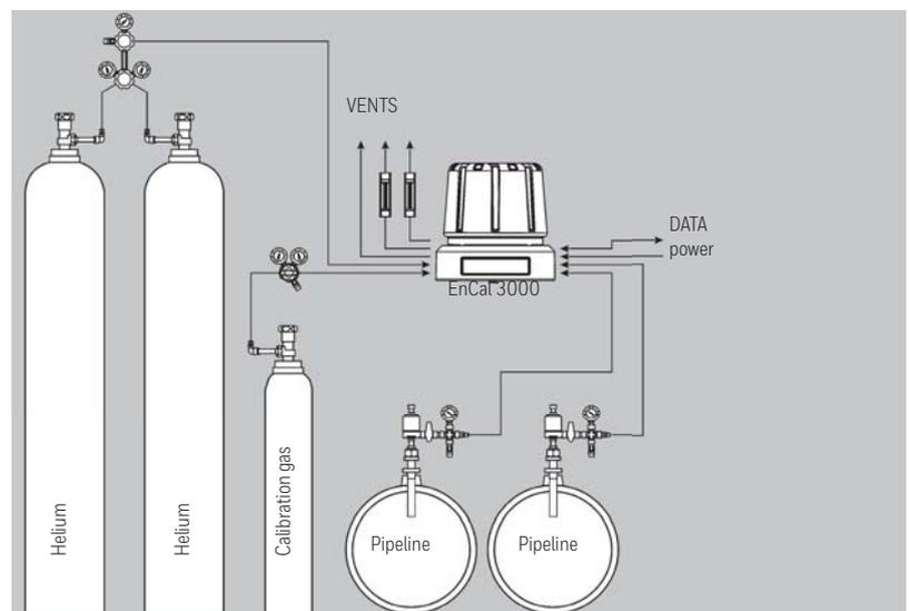
This means that if the analyzer is running several streams in a sequence the next stream to be analysed will be flushed automatically with a flush rate of approx. 0.7 - 1.1 SCF/hr. This is sufficient to flush at least 330 ft of 1/8" sample line.
