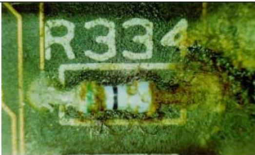
Figure 6 Rodent urine damages components and boards. Sometime the components will actually fall off the board.
