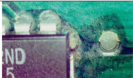
Figure 7 Rodent urine damage results in pin to pin leakage and corrosion.
