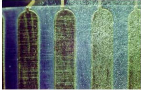
Figure 5 Shown above are card edge fingers covered with dust. A reliable connection is questionable.
