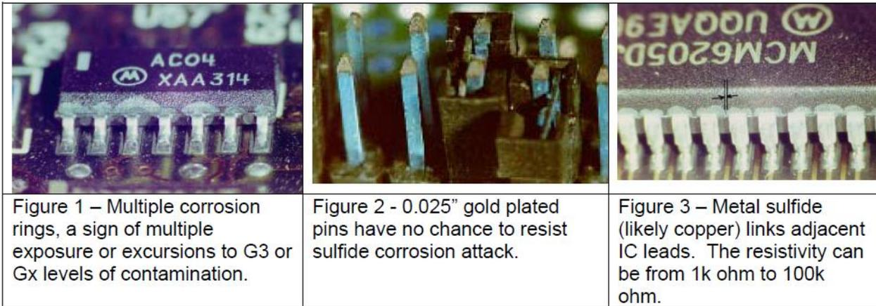
**Hidden mechanism of eCorrosion** can also be detected if you visually scrutinize the surroundings. Three (3) such examples are as follows:
