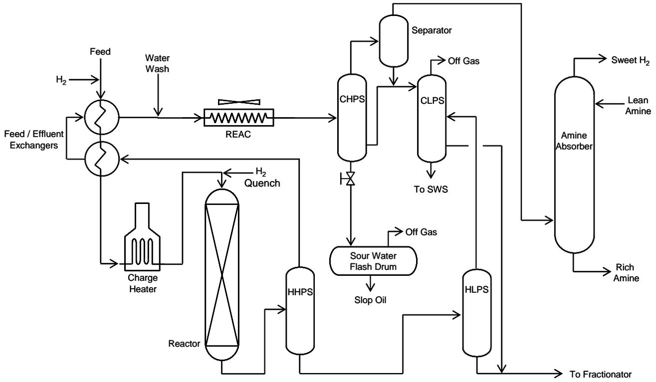
FIGURE 4 – Hydrotreating process flow diagram.
