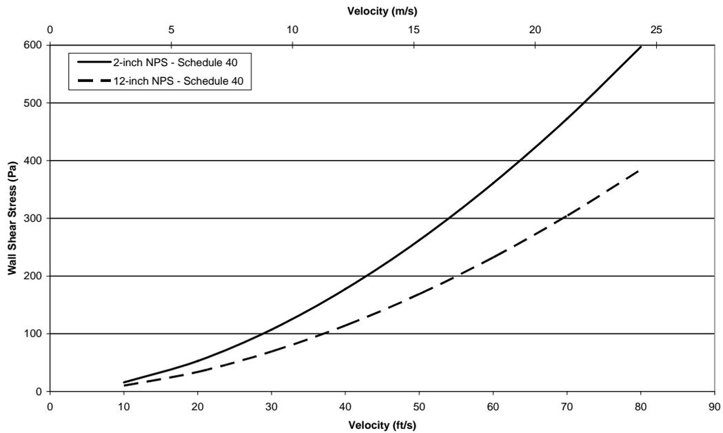
FIGURE 2 – Wall shear stress vs. velocity correlation. [100% liquid flow; 8 wt% NH<sub>4</sub>HS; 130°F (55°C); 50 psia (340 kPa absolute) H<sub>2</sub>S; straight pipe section.]
