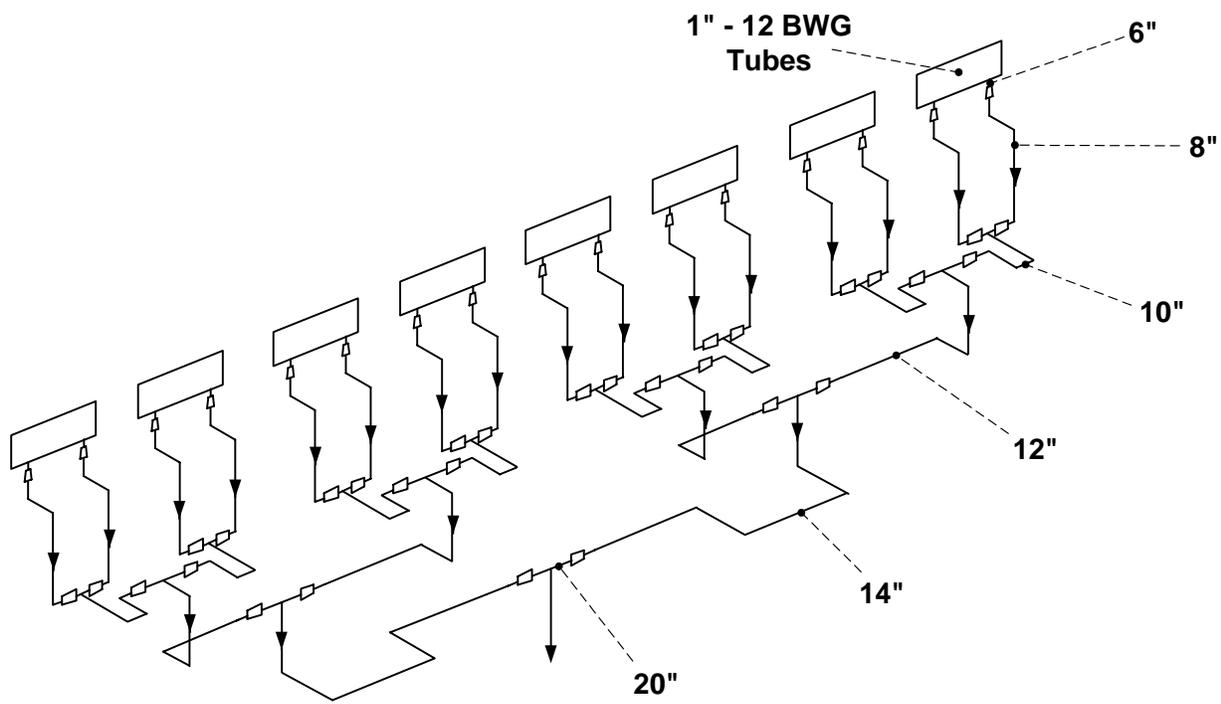
FIGURE 5 – Balanced REAC piping circuit modeled in Hydrotreater B.
