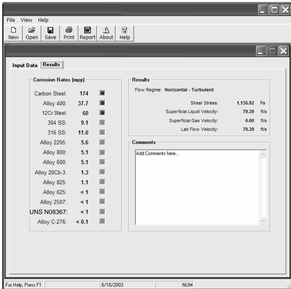
FIGURE 3 – Corrosion prediction software tool results screen.
