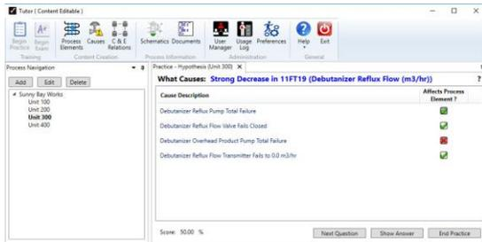
Figure 2. Identifying probable causes of a fault
