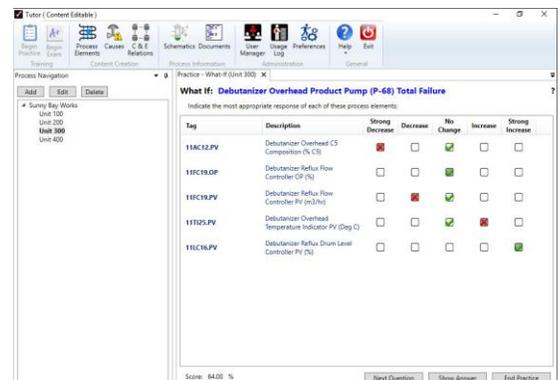
Figure 1. Identifying probable effects of a fault
