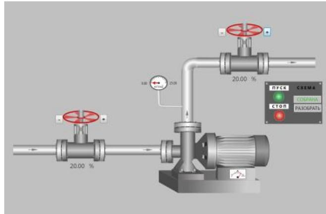
Figure 4. Example of a conventional field operator interface
