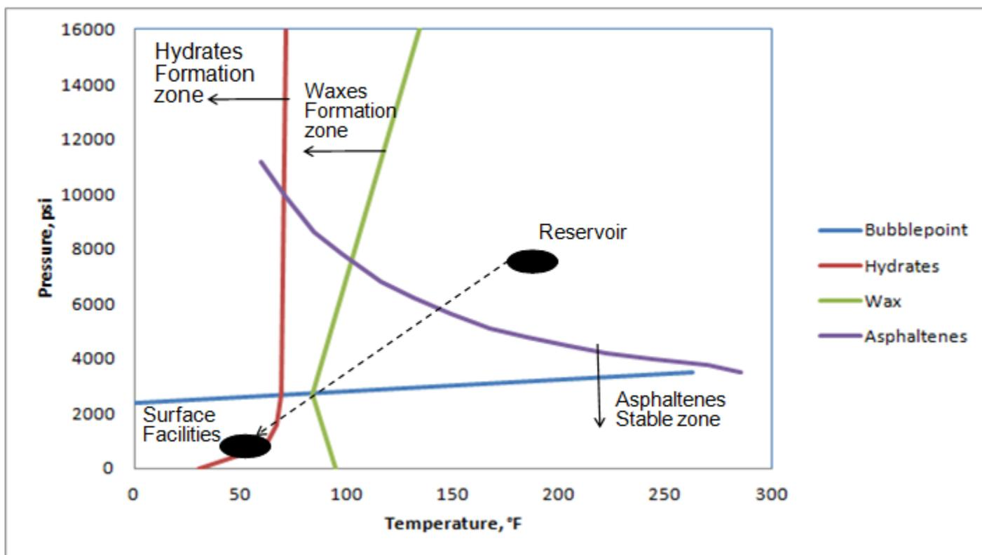
Figure 1. Typical oil-phase envelope, highlighting the hydrates and waxes equilibrium curves, and the asphaltenes precipitation locus<sup>1</sup>.
