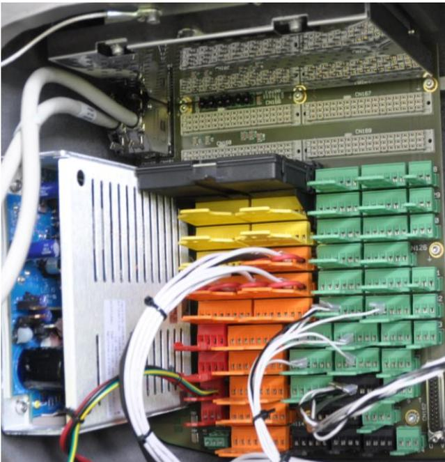
Figure 7. Simplified wiring using a backplane
