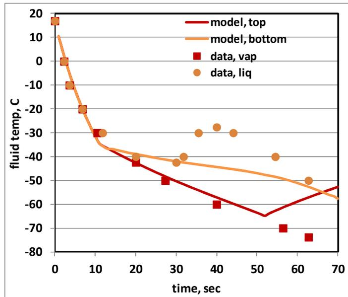
FIG 13. Temperature Profile for Gas 70/30 N<sub>2</sub>/CO<sub>2</sub> blowdown.
