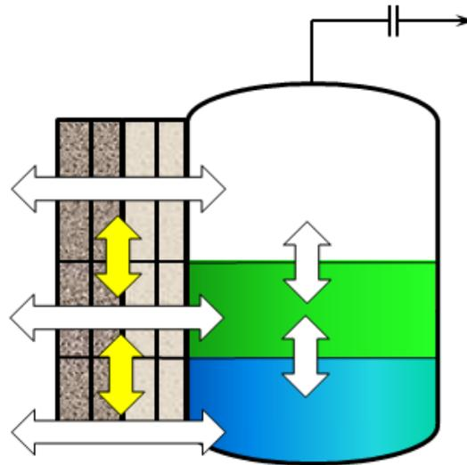
**FIG 4.** Heat-Transfer for Vessel with Three-Phase Non-Equilibrium Model.
