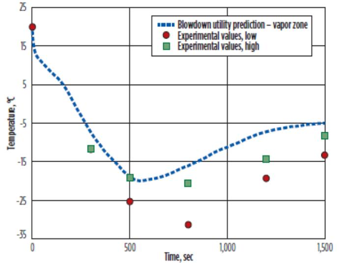
**FIG 7.** Vapour Temperature Profile Spadeadam S12 experiment.
