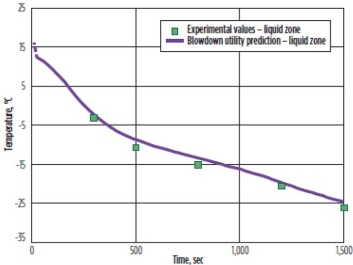
**FIG 8.** Liquid Temperature Profile for Spadeadam S12 experiment.
