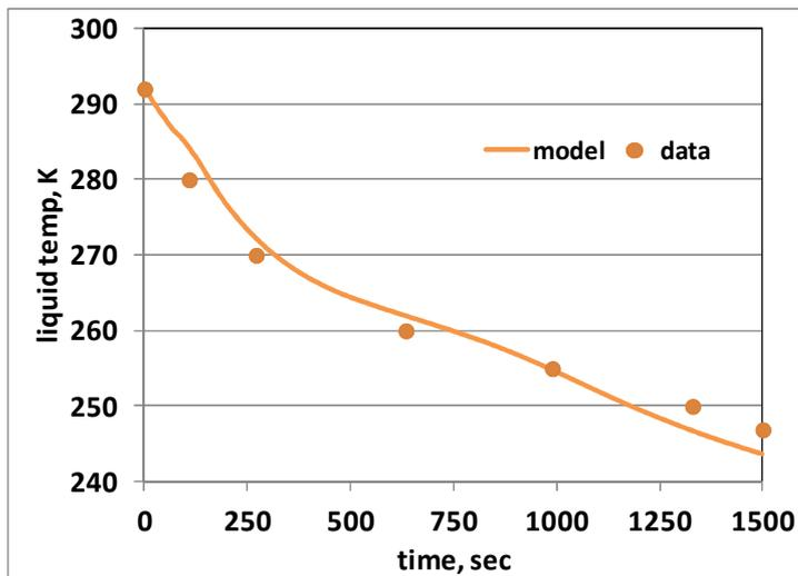
FIG 16. Liquid Temperature for Natural Gas blowdown.
