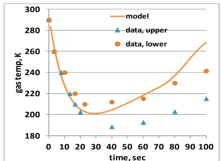
FIG 11. Vapour Temperature Profile for Gas N<sub>2</sub> blowdown.
