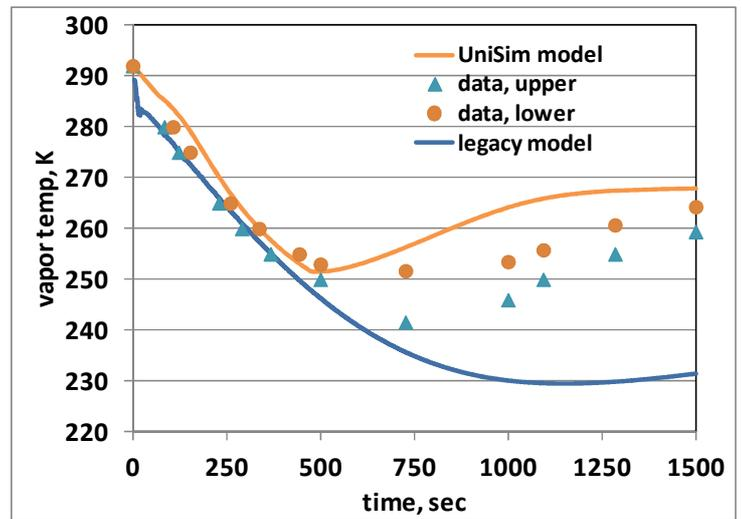
FIG 15. Vapour Temperature for Natural Gas blowdown.
