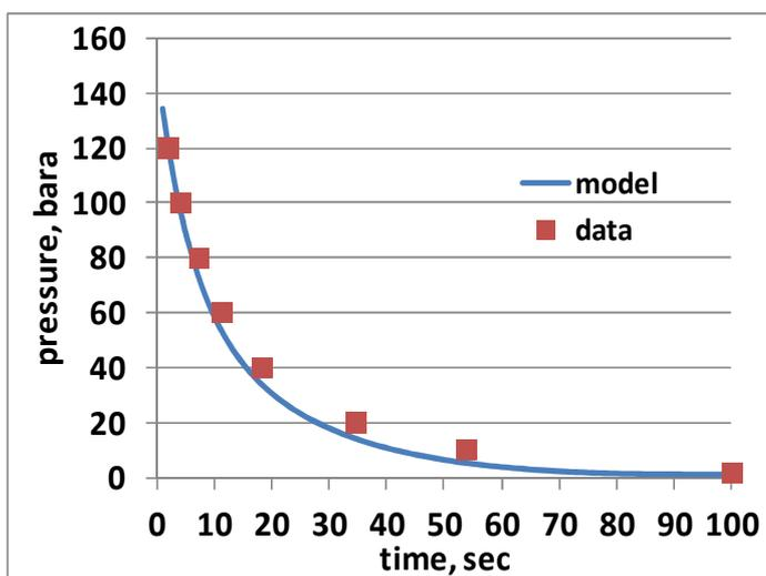
FIG 10. Pressure Profile for Gas N<sub>2</sub> blowdown.
