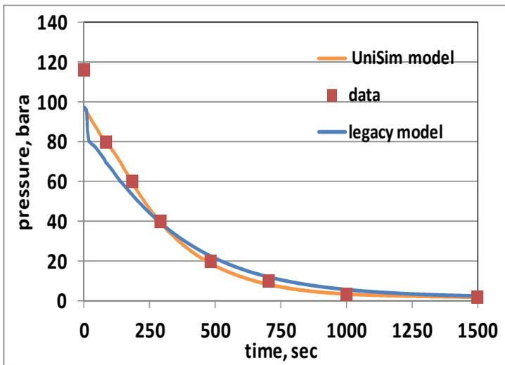
FIG 14. Pressure Profile for Natural Gas blowdown.
