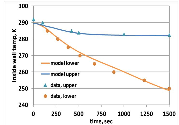
FIG 17. Inner Wall Temperature for Natural Gas blowdown.
