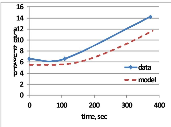
FIG 22. Pressure Profile for Fire Engulfment of LPG test.
