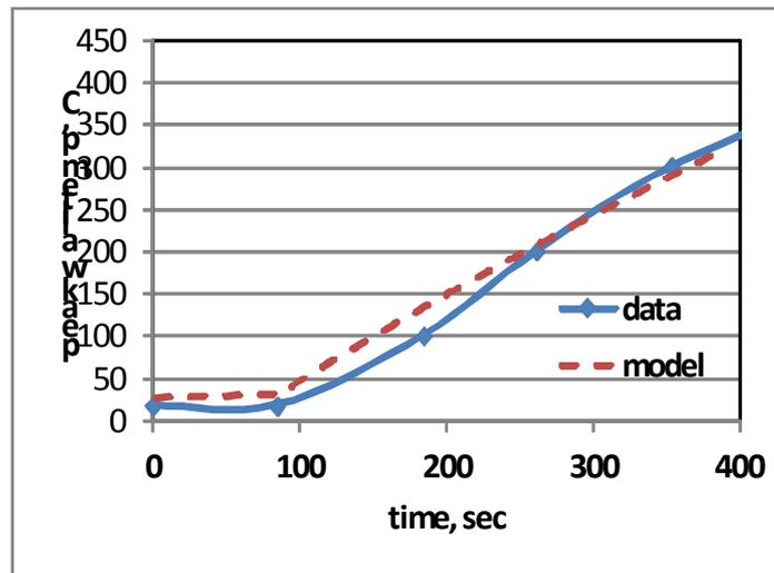
FIG 24. Wall Temperature Profile for Fire Engulfment of LPG test.
