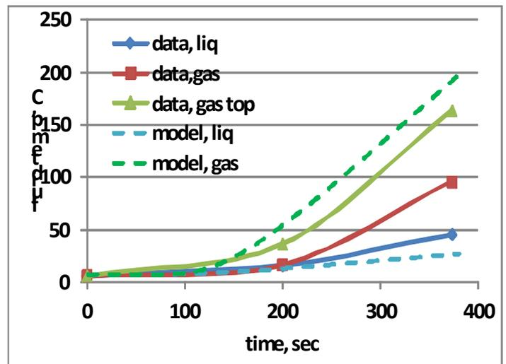
FIG 23. Fluid Temperature for Fire Engulfment of LPG test.
