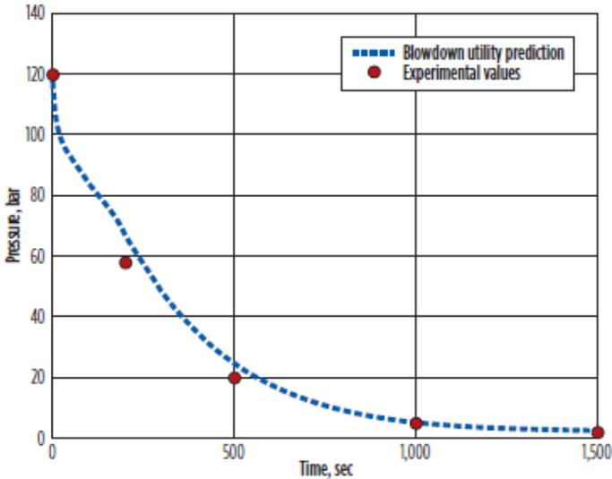
**FIG 6.** Pressure Profile for Spadeadam S12 experiment.
