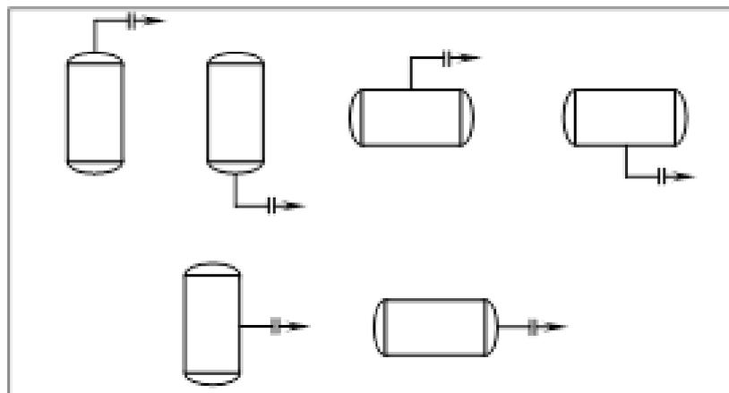
**FIG 5.** Different Vessel Orientations.
