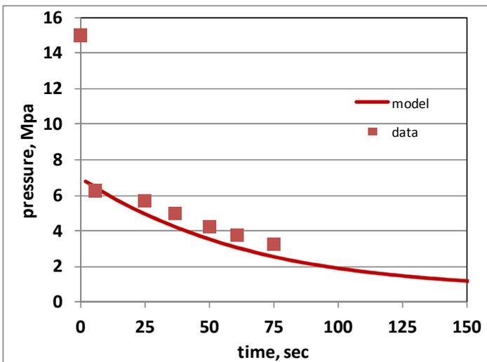
FIG 18. Pressure Profile for Super-Critical CO2 blowdown.
