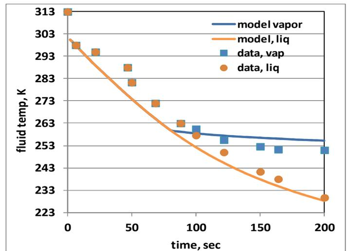
FIG 19. Fluid Temperature for Super-Critical CO2 blowdown.
