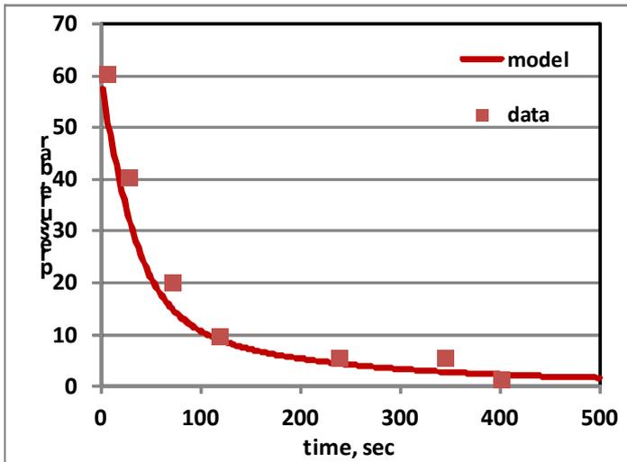
FIG 20. Pressure Profile for Liquid CO<sub>2</sub> blowdown.
