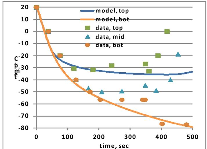
FIG 21. Fluid Temperature for Liquid CO<sub>2</sub> blowdown.
