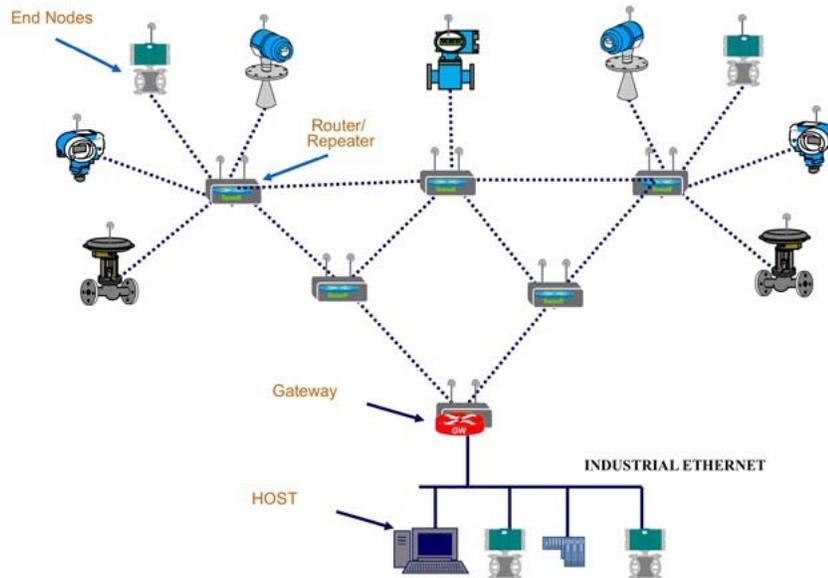
Figure 2. Honeywell's wireless mesh network architecture utilizes externally powered multi-nodes scattered throughout the coverage area.
