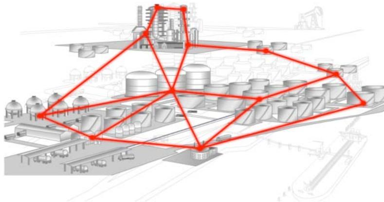
Figure 3. A wireless site survey addressed the coverage area desired at the Gallup refinery, existing power and network infrastructure, and interfering and operating frequencies currently in use or ambient in the environment.
