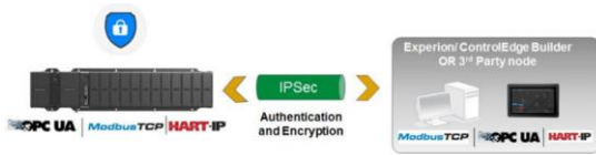
PLC Communication with Experion- Secured with IPSec
