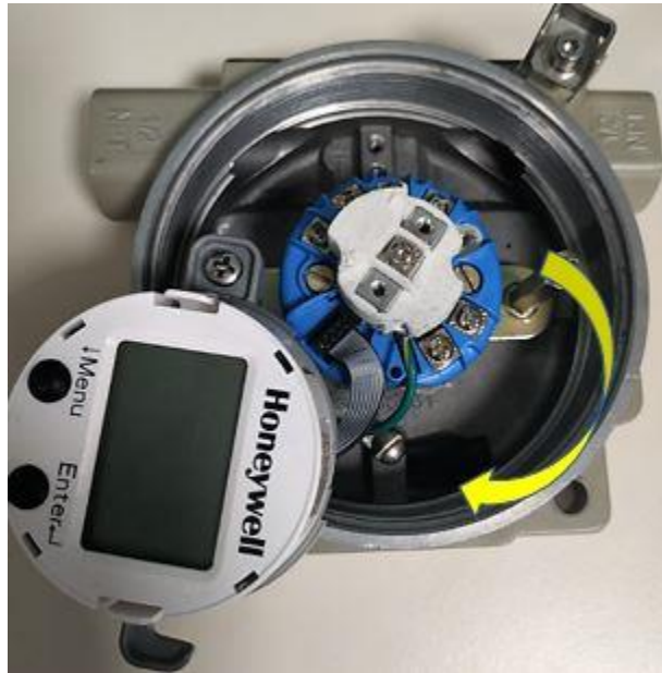
Figure 12: Position of Simple display for external wiring
