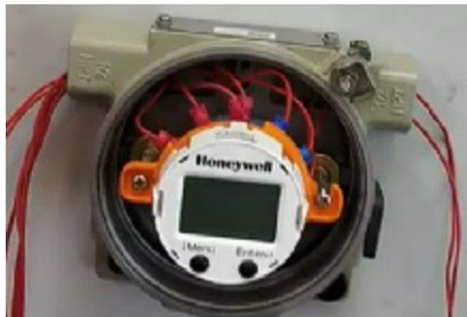
Figure 13: Example of external wiring (Reference only)
