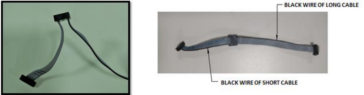
Figure 4: Side view of cable joint (left), Orientation of cables to join (right)
