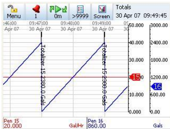
Recorder Trend, Total Printed & Reset every 2 Minutes, aligned to the minute
