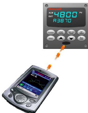
Figure 1-6 Depiction of infrared communications
