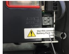
Cloud Link 4G Modem battery connector
